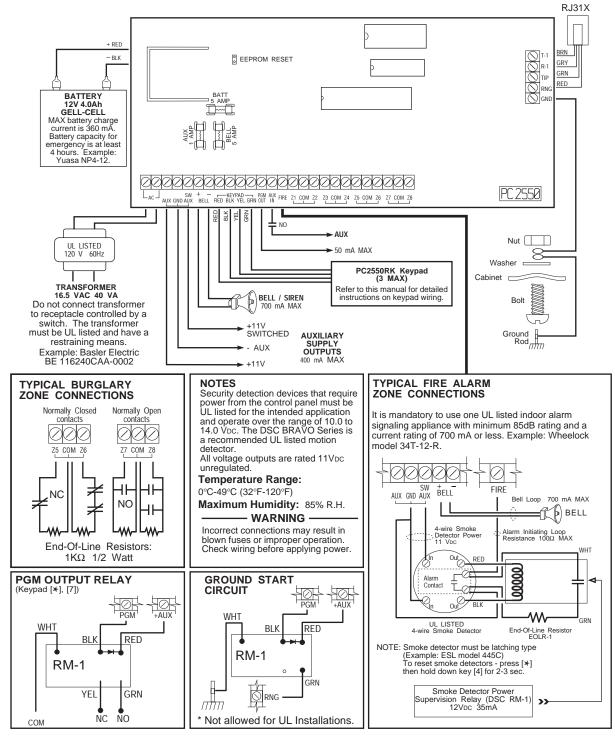
Control Panel is suitable for the following UL installations:
